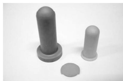
Fig. 2 Appearance of typical proton-conducting oxide: BaCe 0.9 Y 0.1 O 3- \alpha , SrZr 0.9 Y 0.1 O 3- \alpha .
